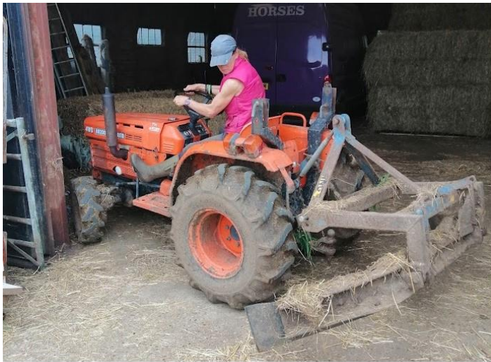
Old scraper on the left with Percy's new rubber bit fitted on the right. We apologise for the emaciated state of Fiona's arms. This is caused by a severe lack of protein, her having been vegan now for some 50 years (hehehehehe)
